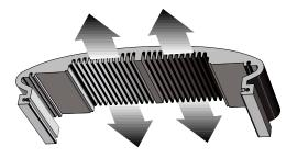
To manage the additional heat associated with higher output capability, a thermally controlled fan has been designed into the *PC4800*. When the heatsink temperature reaches a predetermined value, the fan is activated. Cool air is drawn in through the lower intake vents on the endplate. This cool air flows below the circuit board, through the fan and across the internal fins, cooling the heatsink. The heated air is then forced out through the upper endplate exhaust vents.
